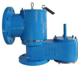
◆ 呼吸閥 ( Pipe Away ) Model: KSBG/GS Size: 2"~14" Set P./V.: +/-22~10,000mmW.C
